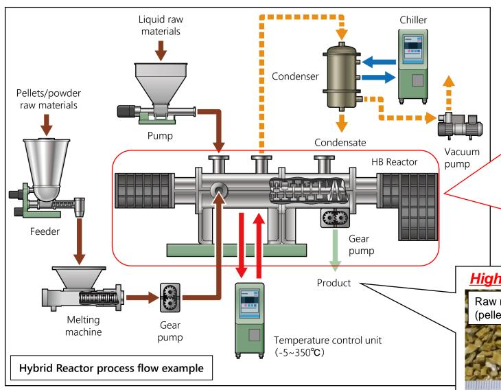
The twin-shaft continuous hybrid reactor has features like "high vacuum", "long residence time" and "high viscosity material handling". It can be used in reaction processes like polymerization (polycondensation), where heat treatment and a long residence time are required.
